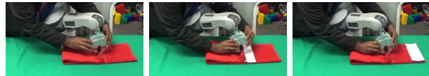
(a) Folding to three fourths of the towel regardless of the placement of the white stripe.
